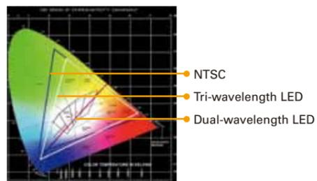
Color gamut enclosed by a tri-wavelength LED is closer to that by a NTSC, which presents delicate and brilliant color, making the after-scanned images as true as the real projects. Therefore, it can capture richer and deeper color than what a two-wavelength LED can do.
